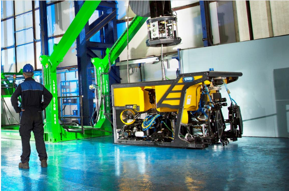
**SMD's Atom MK1 ROV with Hydro-Lek manipulators installed.**
