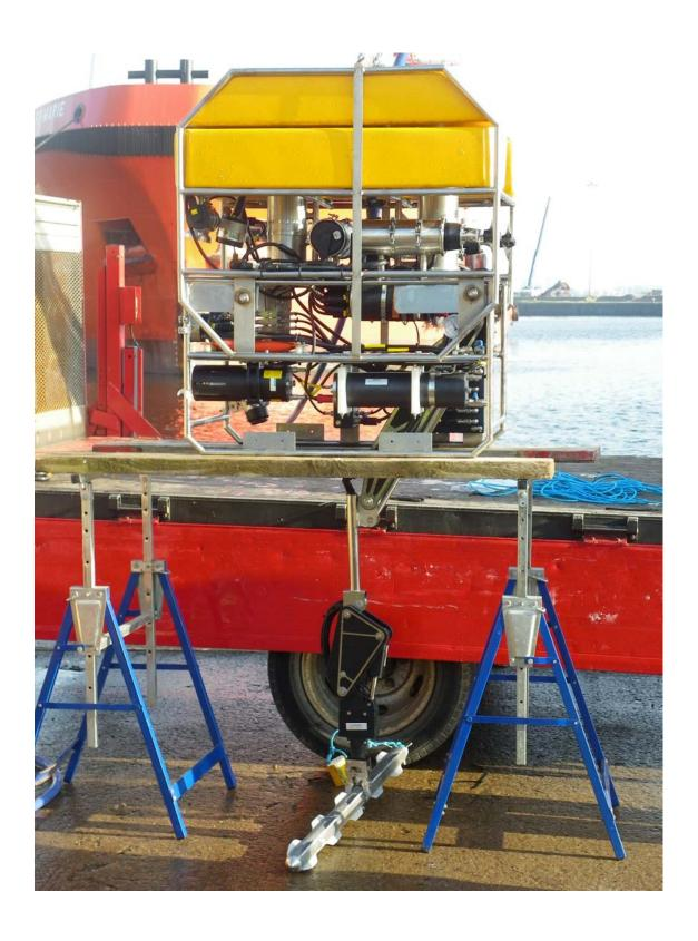
The above picture shows the full reach of the Hydro-Lek 5 function manipulator holding a simulated fuel rod – the manipulator can be retracted fully within the ROV frame.
