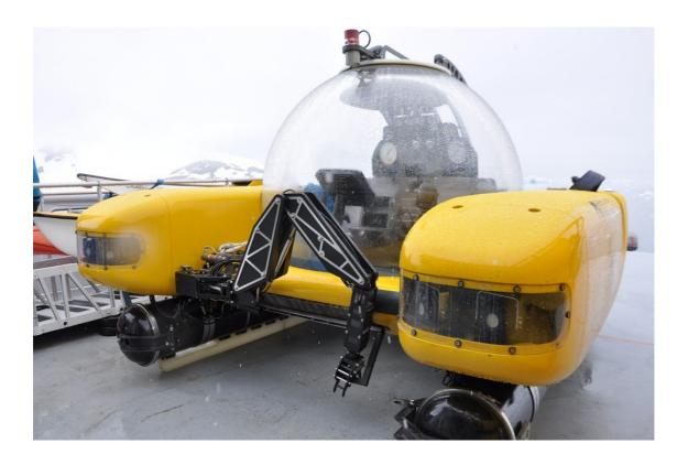
The Hydro-Lek HLK-CRA6 manipulator installed on a Triton 1000/2 Submarine.
