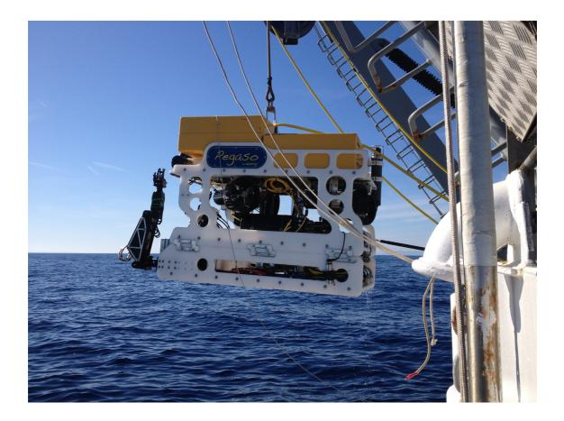
Ageotec's Pegaso ROV complete with Hydro-Lek manipulators for the Italian Navy
