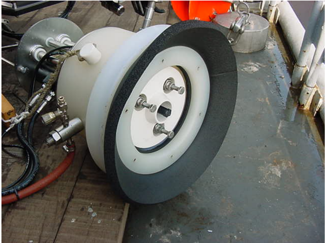
Coffer dam skirt with drill bit and level adjusters
