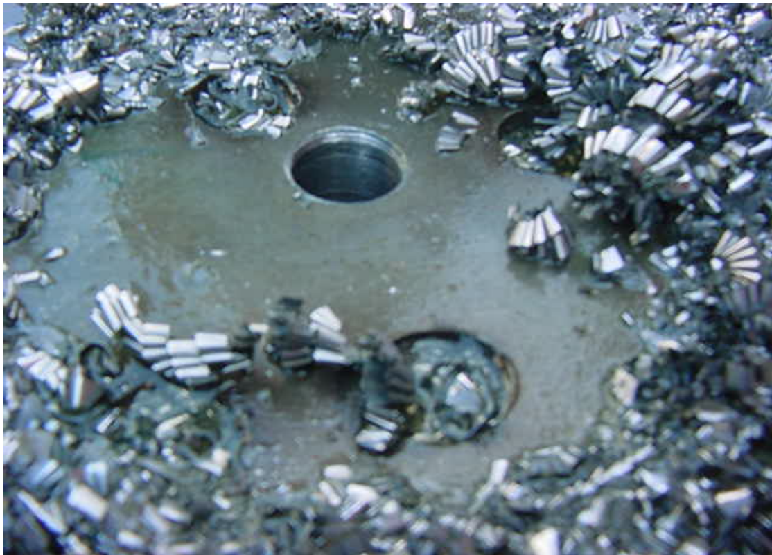
The actual hole size 22 mm after removal of the drill bit
