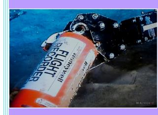
Hydro-Lek's six-function manipulator has been used to successfully recover both flight recorders from the stricken Air France 447 in the Atlantic.
